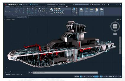
Detail design is a stage in the ship design process that involves creating detailed drawings and specifications for all aspects of the ship. This stage builds on the basic design, and develops a more detailed design that can be used for construction and production.
