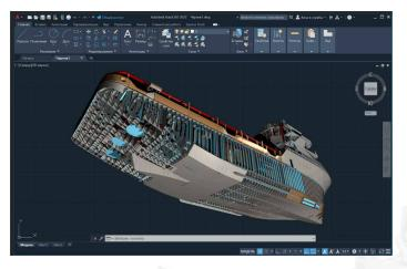
The basic design is a stage in the ship design process that involves creating detailed drawings and specifications of the ship's structure, the propulsion system, and equipment. This stage builds on the conceptual design and feasibility study and develops a more detailed design that can be used for construction.
