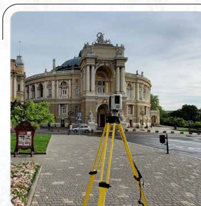
Laser scanning is carried out in order to restore or update the executive documentation, as well as within the framework of the pre-design survey of the reconstruction (repair) object.
